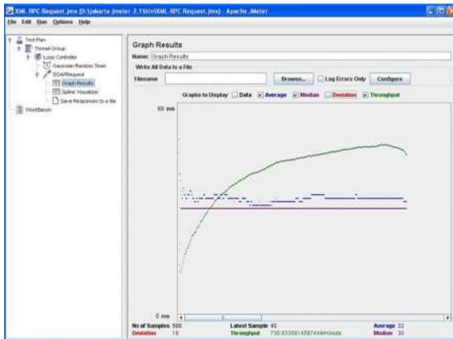
Figure 4. Chart illustrating test results with number of threads = 5, ramp-up time = 10, loop count = 100, and loop controller set to 1 (click the image for a full-size screen shot)
